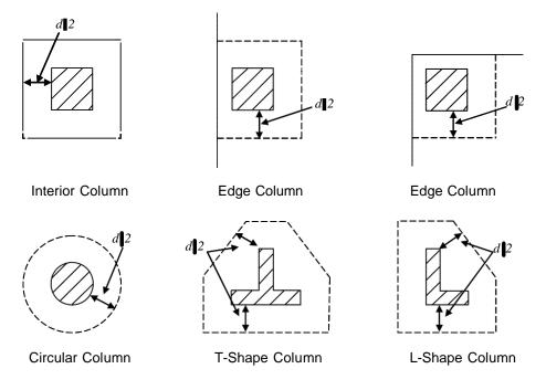
Figure 1-4 Punching Shear Perimeters
