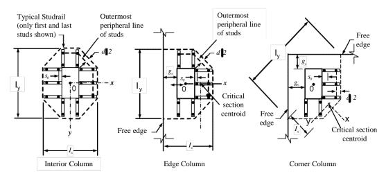
Figure 1-5 Typical arrangement of shear studs and critical sections outside shear-reinforced zone
