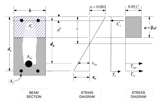
Figure 1-1 Rectangular Beam Design
