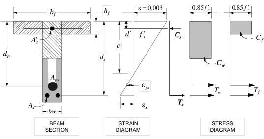
Figure 1-2 T-Beam Design
