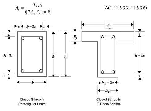
Figure 1-3 Closed stirrup and section dimensions for torsion design
